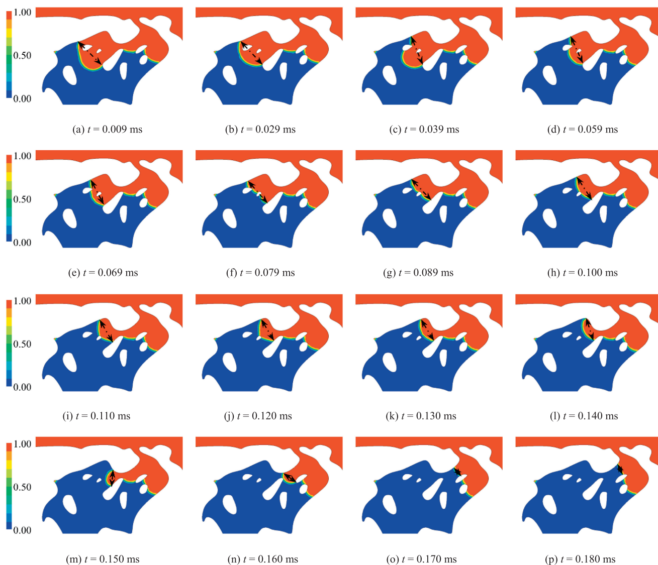
Fig. 17. The dynamic changing of the liquid front end in the pores.
